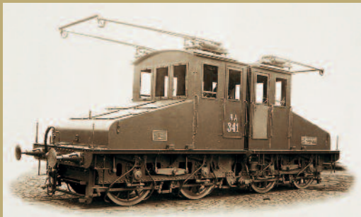
The Valtellina railroad's engine. It was designed by Kálmán Kandó and made by the Ganz factory. With this, the alternate-current electrification of railroads have begun in the world.
