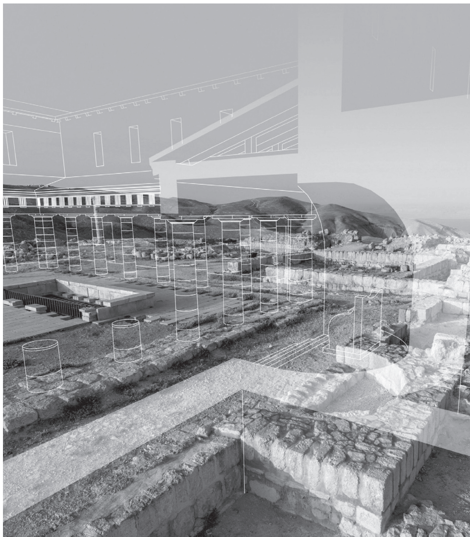
Fig. 25: The theoretical architectural reconstruction of the Herodian throne seat, superimposed on a photograph of the surviving and conserved ruins; cutaway view from north.
